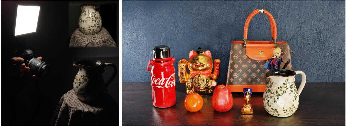
Fig. 1. Our inverse rendering system captures both the BRDF material and geometry of real-world objects using active area lighting. Leveraging differentiable LTC, the area lighting provides a broader range of BRDF samples while maintaining rendering efficiency similar to a single point light. This enables fast, high-fidelity inverse rendering, allowing for accurate renderings of novel views under various lighting conditions.
